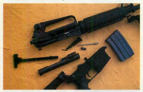
Fieldstripping just like the Military M4 Carbine, the Bushmaster comes apart and goes back together in minutes without the need for tools. (below) Bushmaster carbines with removable carrying handles will accept the new Selective Integrated Rail (S.I.R.) System now being tested by the U.S. Special Operations Command (SOCOM). A commercial version of the S.I.R. System will soon be available.
